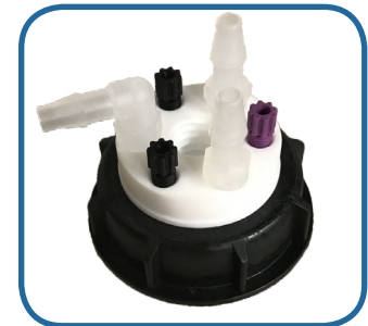
SW55-3-C-3L : 3 entries 1/8", a charcoal cartridge emplacement and 3 threaded barbed fittings
