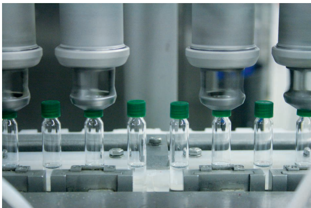
Automatic fastening of the cuvette caps
