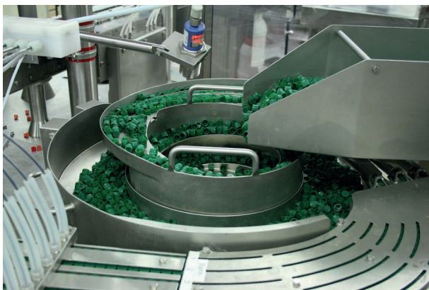
Preparation of the cuvette caps in the control and sorting drum.
