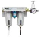
The 2-stage air filtration assembly consists of a Balston Grade DX coalescing filter and a Balston Grade BX coalescing filter. Together these filters remove oil, water and particulate contamination (99.99% at 0.01 micron) from the compressed air supply.
