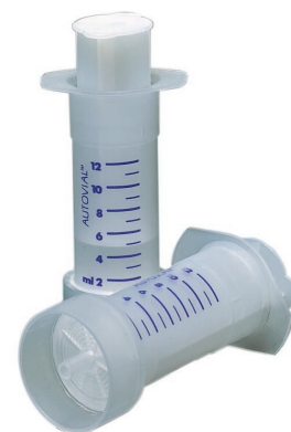
Fig 17: Autovial 5 syringeless filter.
