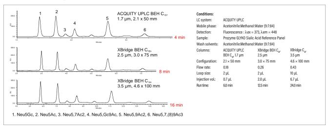
Geometric scaling of DMB-labeled sialic acid standards on XBridge BEH C<sub>18</sub>, 130Å, 3.5 µm particle (bottom), 2.5 µm particle (middle), and ACQUITY UPLC BEH C<sub>18</sub>, 130Å, 1.7 µm particle (top).
