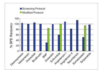
The innovative Oasis µElution Plate format allows for as much as a 15-fold increase in the concentration of sample, increasing the possibility of reaching the required sensitivity levels for bioanalytical assays. The low, 25 µL, elution volume eliminates the need for evaporation and reconstitution, significantly reducing the potential loss of analyte by its adsorption to the walls of the collection plate, chemical instability, or both.
