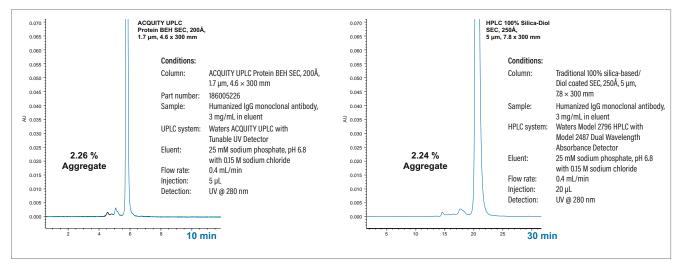
Compared with traditional HPLC-based SEC technology, Waters ACQUITY UPLC BEH SEC Technology delivers a comparable determination of mAb aggregate vs. monomer content in significantly less time, promoting higher sample throughput.
